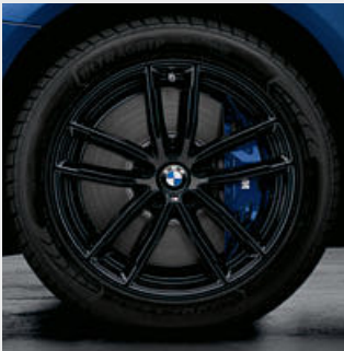
○ High-quality 18" M light alloy wheel Double-spoke style 662 M in Jet Black. TPMS winter complete wheel with run-flat tyre.
